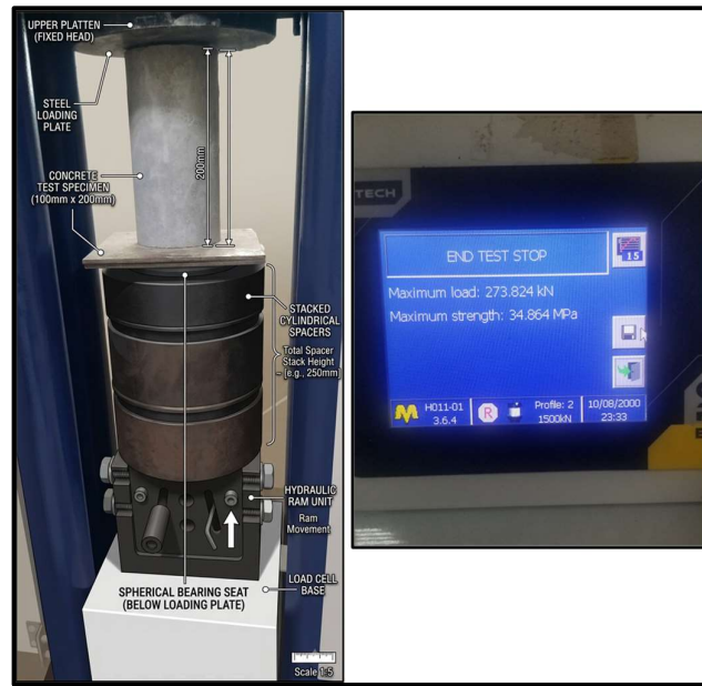
Figure 5, Compressive Strength Test Set-Up
